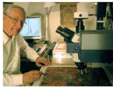
Raman microscope for Tibetan scroll paintings
